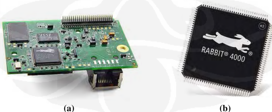
Gambar 2.1. (a) Modul RCM4300 (b) Mikroprosesor Rabbit 4000 [7]
