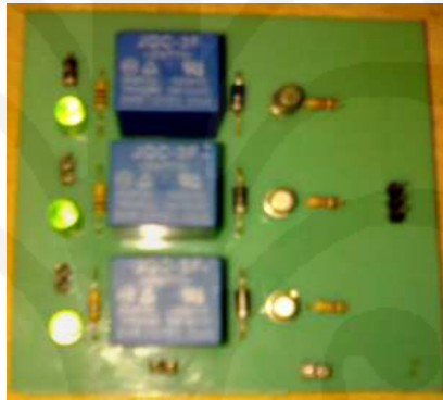
Gambar 4.1 Modul Driver Heater dan Driver Blower
