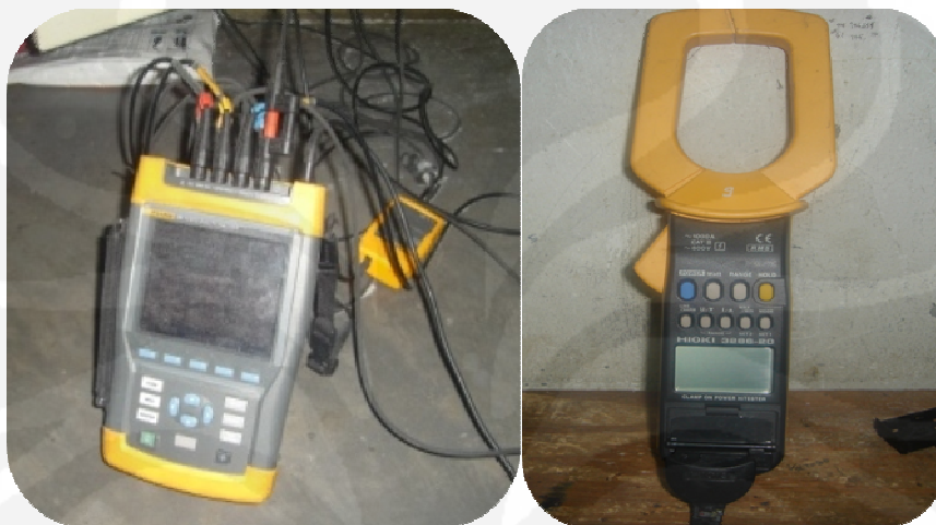
Gambar 3.3. Power Analyzer dan Clamp on
