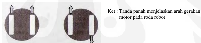
Gambar 2.2 Sistem Gerak Differential Drive
