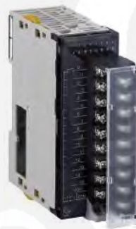
Gambar 2.12 PLC Input CJ1W-ID211
