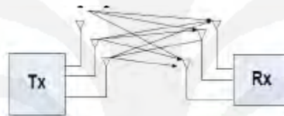
Figure 1 Array of antenna in MIMO
