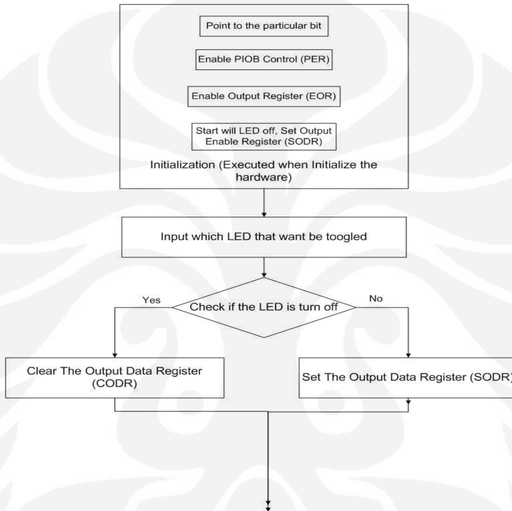
Figure 25 - Algorithm to toggle the LED
