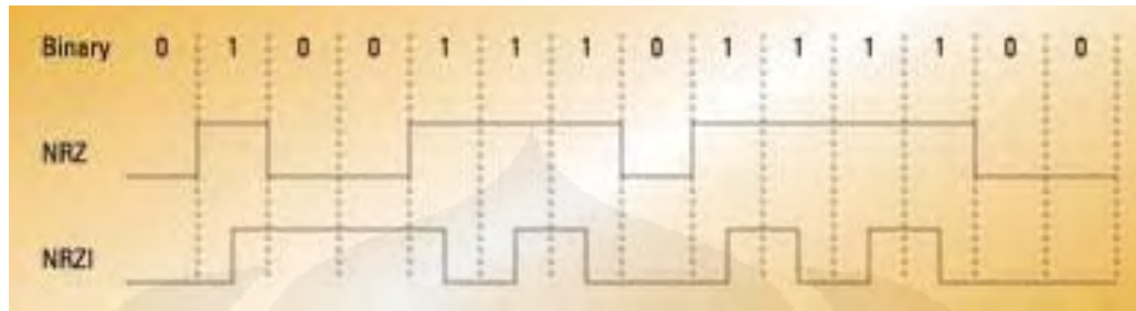
Figure 7 - NRZ to NRZI Encoding Example
