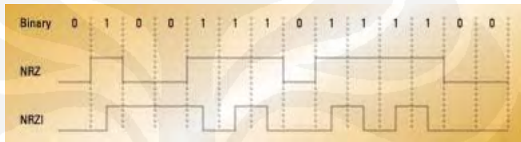
Figure 7 - NRZ to NRZI Encoding Example
