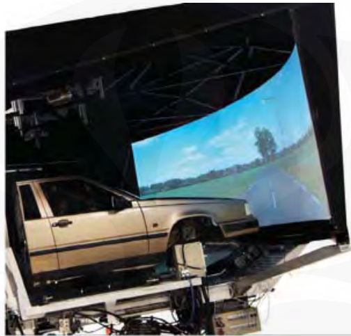
Gambar 2. 2: The VTI Driving Simulator III Sumber: Swedish National Road and Transport Research Institute (2004)
