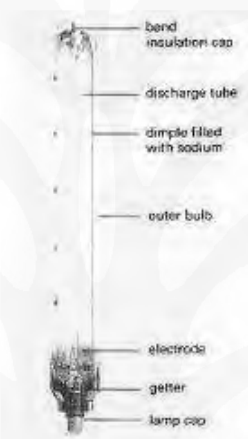
Gambar 3. 8 Bagian Lampu Low-pressure Sodium
