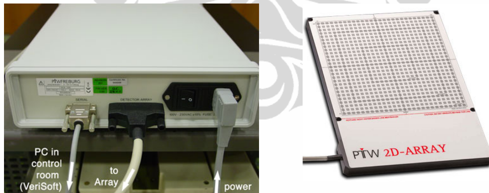
Gambar 3.1 (a) Sisi belakang interface, (b) PTW 2D array 17
