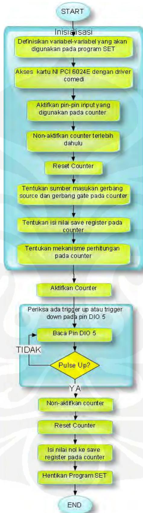
Gambar 3.6 Diagram Alir Algoritma Program SET
