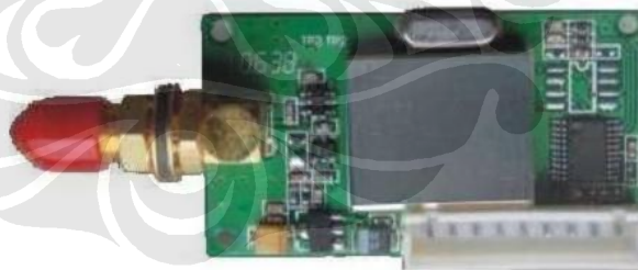
Gambar 2.7. Modul wireless YS-1020UA RF Data Transceiver
