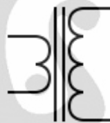
Gambar 2.10 Skema transformator step up
