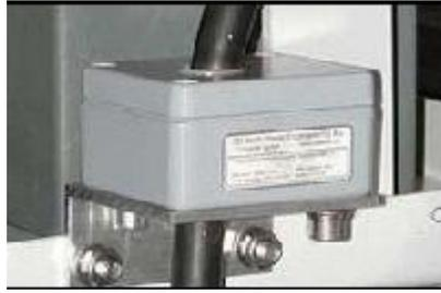
Gambar 3.4 High Frequency Current Transformer
