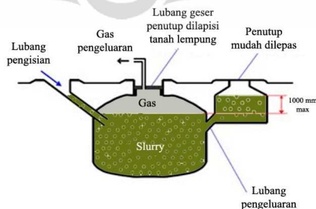
Gambar 2.7 Digester tipe fixed dome (China)
