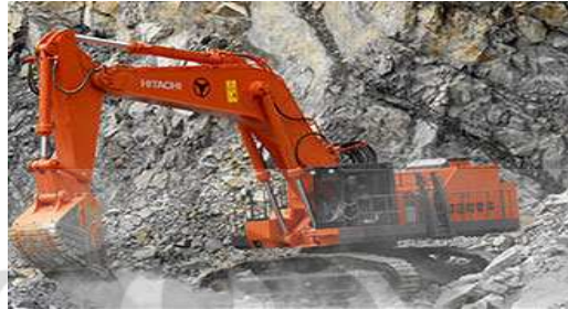
Gambar 3.4 Excavator Tipe EX1200
