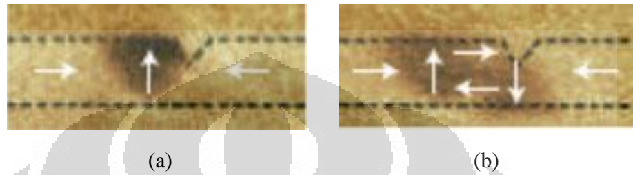
Figure 2.6 Magnetic structure of permalloy nanowire observed using MFM (a) transverse DW structure, (b) vortex DW structure [3].
