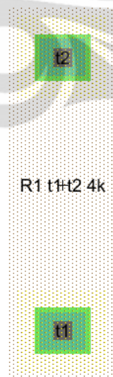
Gambar 4.22 Layout n-well resistor
