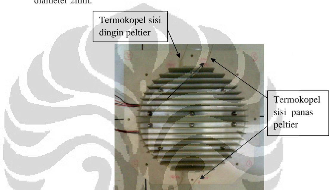
**Gambar 4.5** Posisi thermokopel peltier
