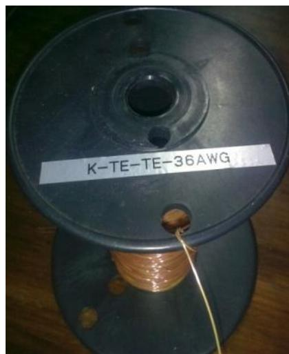
Gambar 3. 14 *Thermocouple* Tipe K
