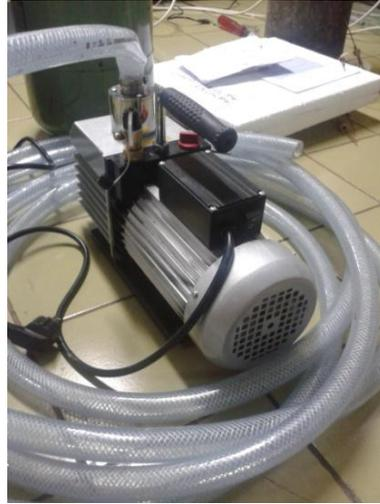
Gambar 3.4 Pompa Vakum
