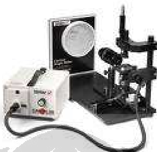
Gambar 3.5 Contact angle meter ( www.wikipedia.org , 2009)
