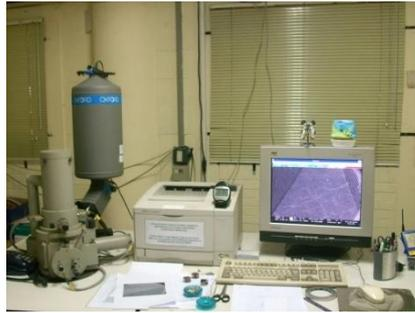
**Gambar 3. 4 Alat SEM (Scanning Electron Microscopy)**
