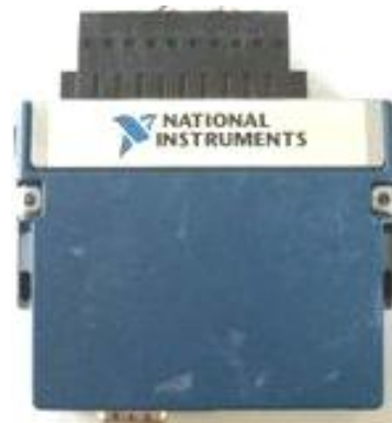
Gambar 4. 11 Modul National Instrument tipe 9211
