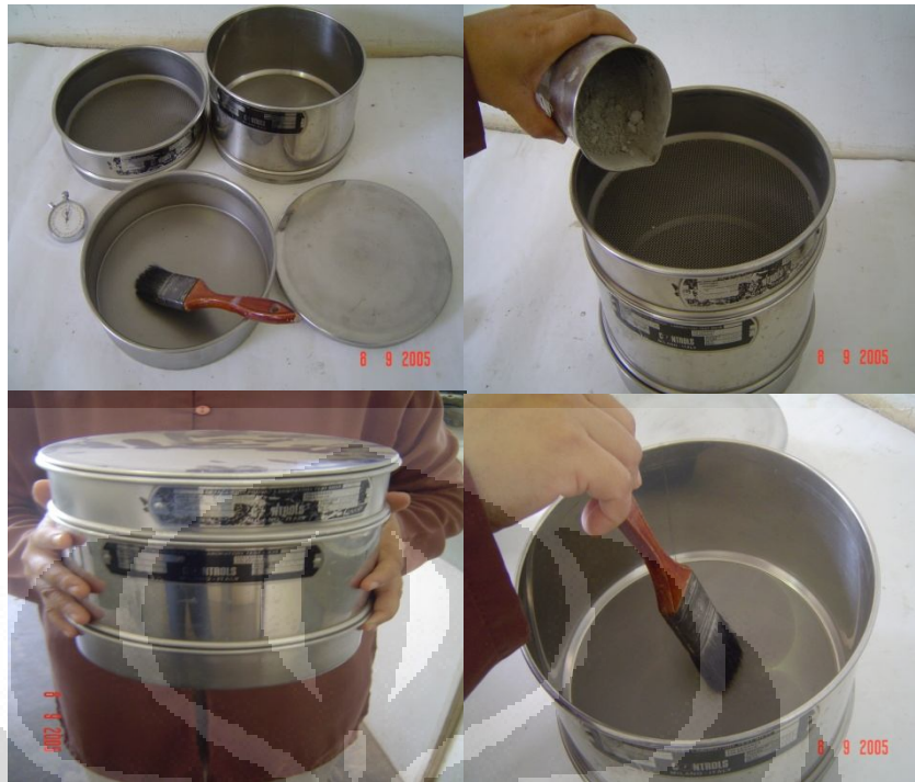
Gambar 3.3 Prosedur Pengujian Analisa Ayak
