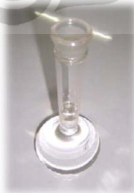
Gambar 3.5 Alat pycnometer uji specific gravity
