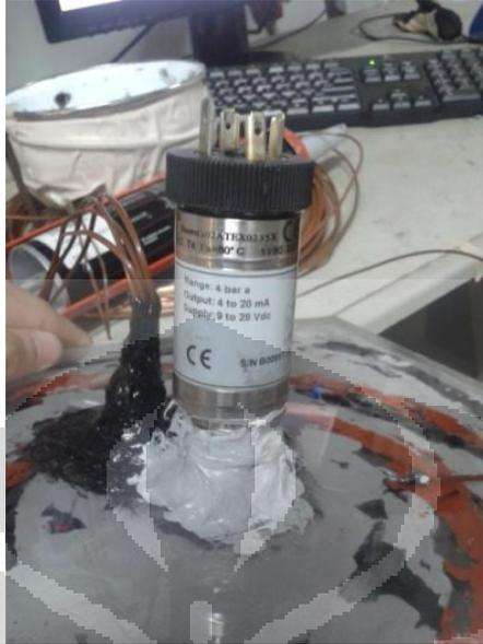
**Gambar 3.13.** *Pressure Transmitter*
