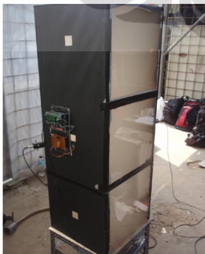
Gambar 4.5. Ruang uji adsorpsi gas CO
