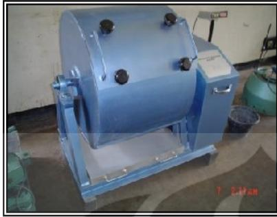
Gambar 3.6 Mesin *Los Angeles*
