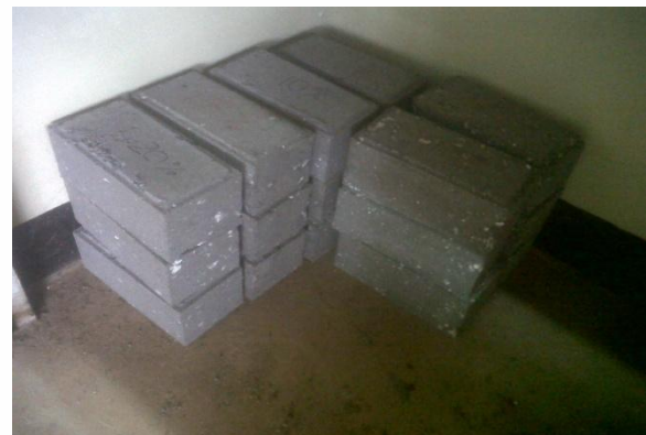
Paving Block Pasca Pencetakan
