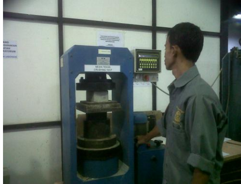
Gambar 3.2. Mesin uji tekan beton / paving block
