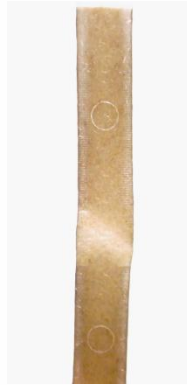
Figure 4. 8 Failure mode of compressive specimen test flax/PP
