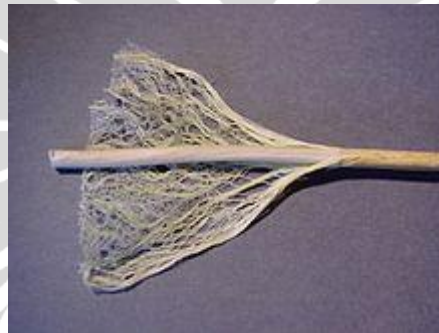
Figure 2. 6 Dried hemp stalk showing outer bast fibres and inner core or stick fibres
