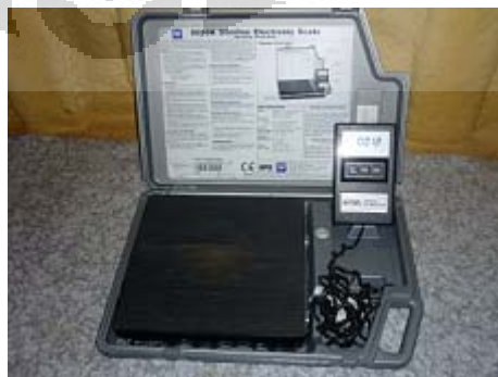
Gambar 3.7. Electronic Refrigerant Scale
