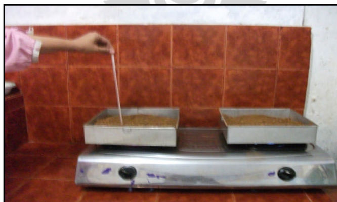
Gambar 3.2 Pemanasan Sampel ( T = 150^\circ\text{C} , t = 6 jam)
