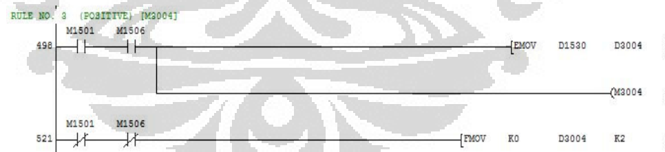
Gambar 3.46 Pemrograman aturan fuzzy no. 3
