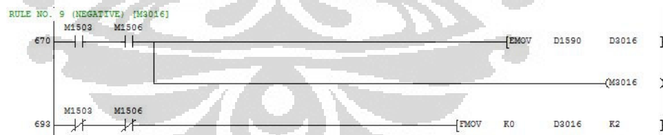
Gambar 3.52 Pemrograman aturan fuzzy no. 9
