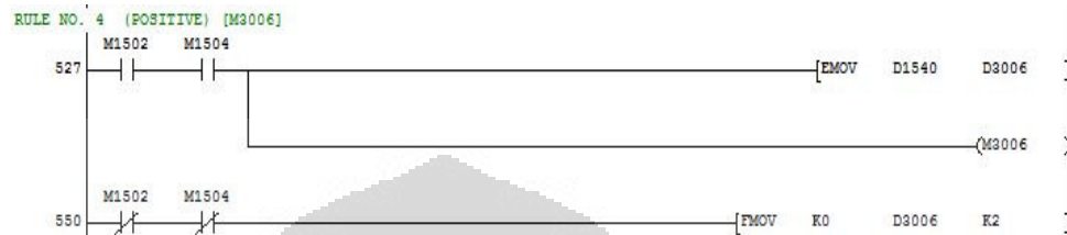
Gambar 3.47 Pemrograman aturan fuzzy no. 4
