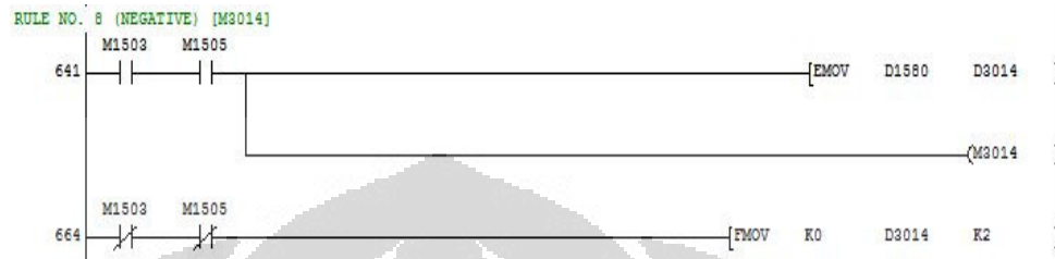
Gambar 3.51 Pemrograman aturan fuzzy no. 8
