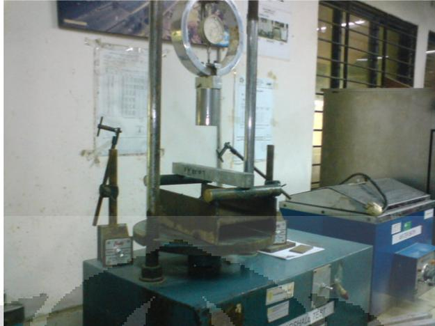
**Gambar 3.8.** Mesin Uji tarik Lentur (*Flexural Strength Testing Machine*)
