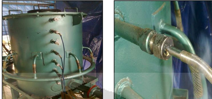
Gambar 3.8 Thermocouple tipe K
