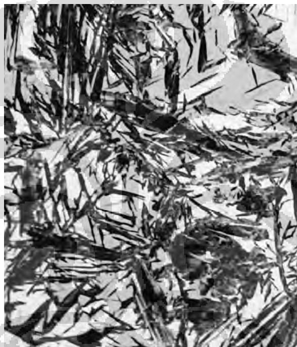
Gambar 2.6 Fotomikro Lath Martensit hasil Quench [13]
