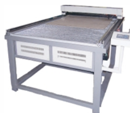
Gb 2.6 Mesin wide laser cutting [10].
