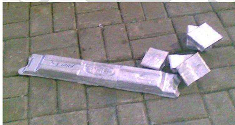
Gambar 3.15 Ingot aluminium paduan AC4B
