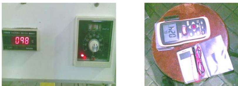
Gambar 3.21 Termokontroller, termokopel fix & portable.
