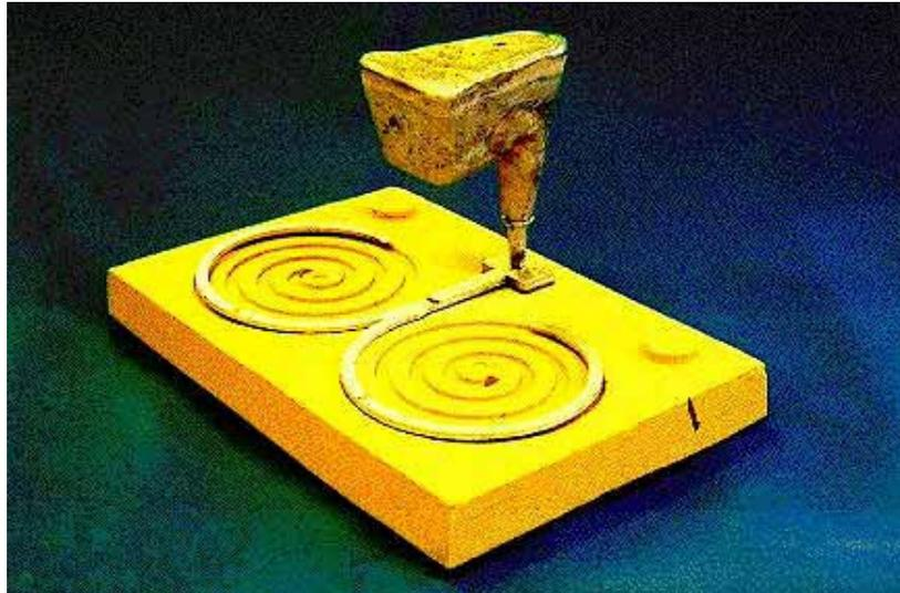
Gambar 3.5 Alat uji fluiditas gravitasi spiral (*original methode*) [3]
