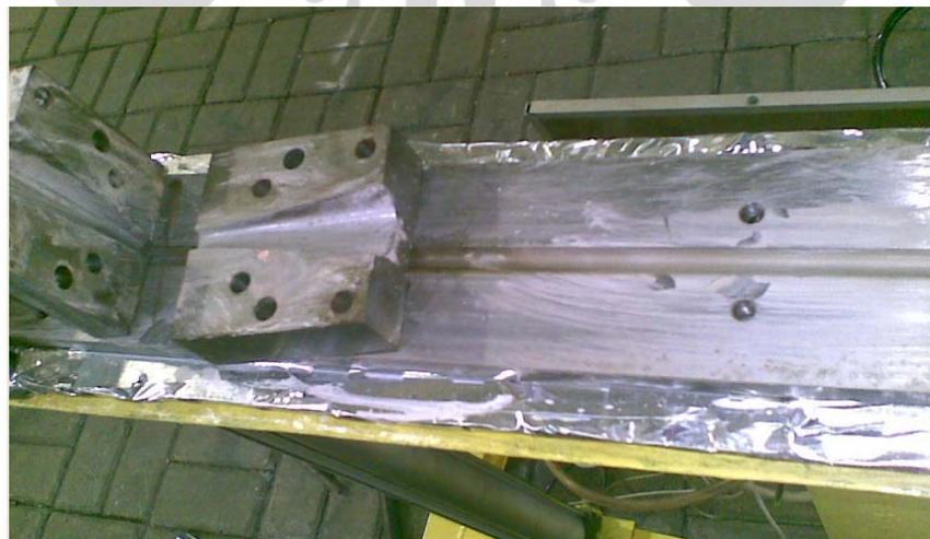
Gambar 3.17 Hasil proses *coating* zircon
