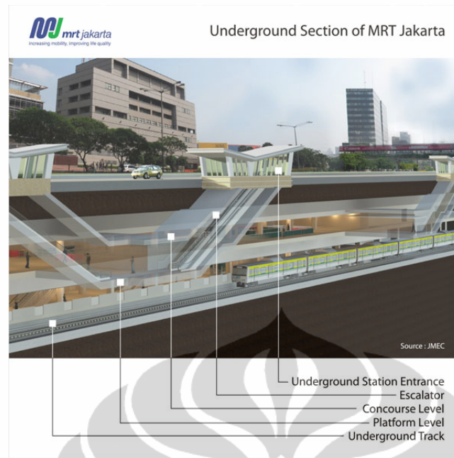
Gambar. 4.3 Underground Station , Sumber: PT. MRT Jakarta
