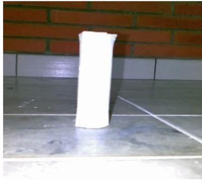
Gambar 4.1 Prekursor hasil *slip casting*.
