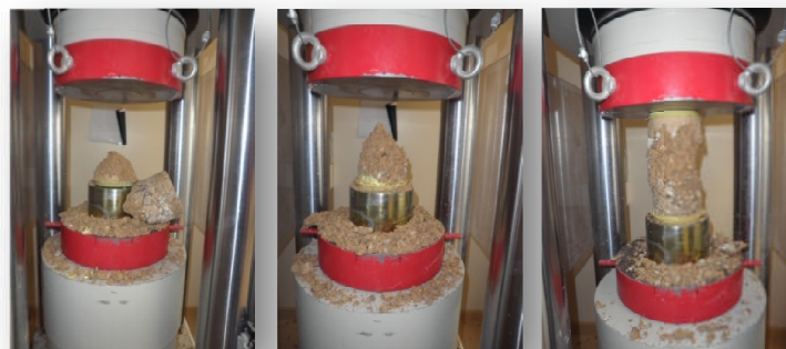
Figure 4.6 Compressive Strength Test 28 th Day Mix#2
