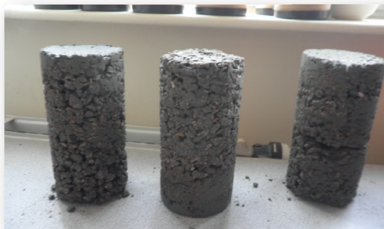
Figure 5.3 Hardened Mix#3 at 7 th day before Compressive Strength Test
