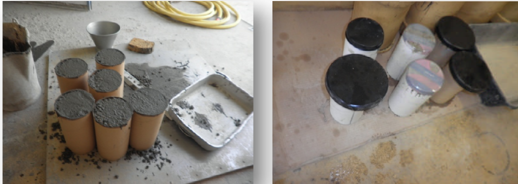
Figure 3.6 Casting Specimen 11x22 cm for Compressive Strength
