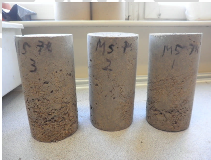
Figure 5.4 Hardened Mix#4 at 28 th day before Compressive Strength Test
