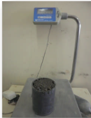
Figure 3.10 Weighing Density of Fresh CLSM
