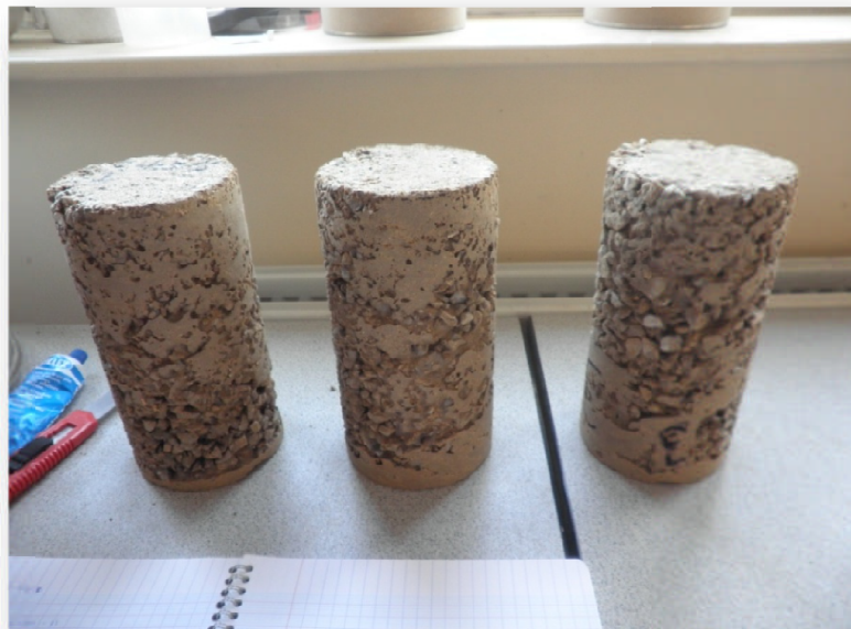
Figure 5.2 Hardened Mix#2 at 7 th day before Compressive Strength Test
