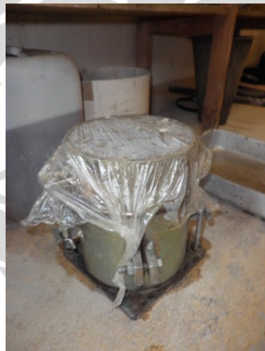
Figure 3.7 Casting Specimen 15x20 cm for IPI Test
