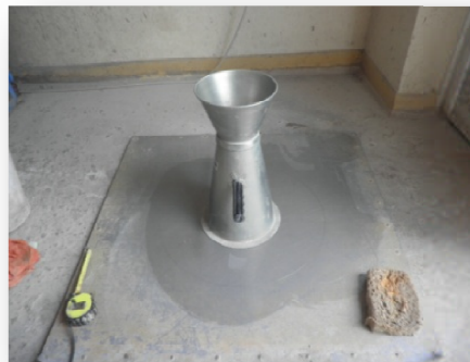
Figure 3.9 Slump Flow Test Equipment
