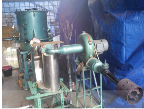
Gambar 3.15 Fixed Bed Downdraft Gasifier
