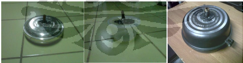
gambar 3. 5 wadah material ( material tray ) stainless steel , plastik, teflon
