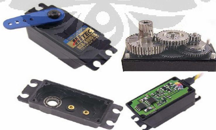
**Gambar 2.5** Sistem Mekanik Motor Servo[3]
