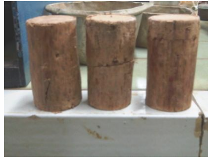
Gambar 3.13. Sample Tanah Hasil Triaxial UU Test
