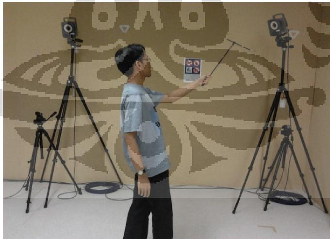
**Gambar 3.14** Proses Kalibrasi Dengan *Wand*
