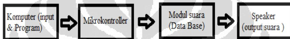
**Gambar 3.1 Blok diagram Alat**
