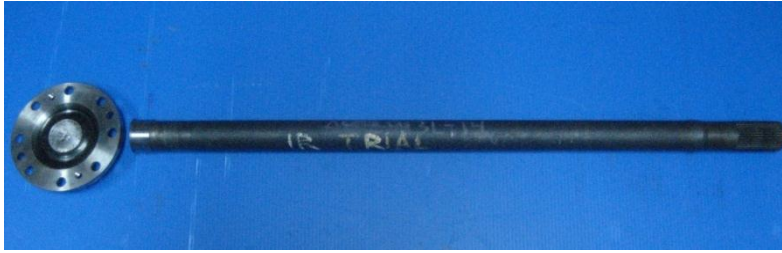
Gambar 2.4 Axle Shaft patah
