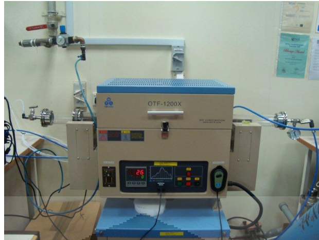
Gambar 3.1 Mesin Furnace MTI
