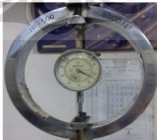
Gambar 4.3 Proving ring saat dibebani
